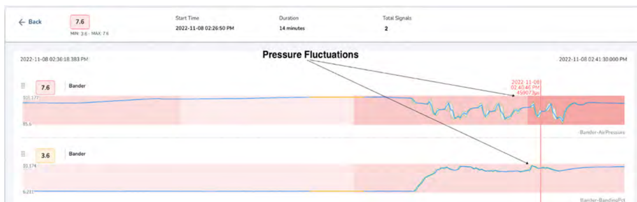
Figure 5. Example 1: Pressure fluctuations in a downcoiler bander.
